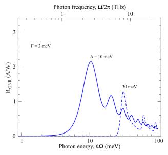
Fig. 6. Responsivity of GNR photodiodes with different values of the energy gap ( $\Delta = 10 \text{ meV} - \text{solid curve}$  and  $\Delta = 30 \text{ meV} - \text{dashed curve}$ ) as a function of the photon energy and frequency at  $\Gamma = 2 \text{ meV}.$
