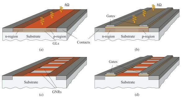
Fig. 2. Schematic views of MGL p-i-n photodiodes with (a) chemically doped p- and n-regions and (b) electrically induced p- and n-regions (electrical doping), as well as of GNR p-i-n photodiodes with (c) chemically doped p- and n-regions and (c) electrically induced p- and n-regions, respectively. A circuit example (for an MGL photodetector with electrically induced p- and n-regions) is shown in Fig. 3(a).
