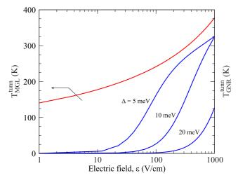
Fig. 10. Electric field dependences of characteristic temperatures  $T_{MGL}^{tunn}$  (left scale) and  $T_{GNR}^{tunn}$  (right scale) for different energy gaps  $\Delta$ , corresponding to resonant frequencies  $\Omega/2\pi = \Delta/2\pi\hbar = 1.27, 2.54$ , and 5.09 THz, respectively. The areas above and below the pertinent curve correspond to dominating thermogeneration and tunnelling dark current mechanisms, respectively.
