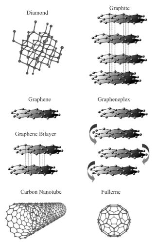
Fig. 1. Schematic view of carbon structures: 3D diamond and graphite; 2D – graphene, graphene bilayer, and multiple graphene structure with disoriented layers (grapheneplex); 1D – carbonnano-tube; 0D – fullerene (C<sub>6</sub>0). Arrows at graphene-plex structure indicate disorientation (twist) of non-Bernal stacked graphene layers.
