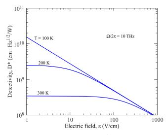
Fig. 9. MGL photodiode detectivity for  $\Omega/2\pi = 10$  THz as a function of the electric field at different temperatures.
