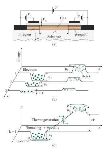
Fig. 3. (a) Structure of MGL photodiode with electrically induced pand n-regions and the pertinent wiring, (b) energy band diagrams of GLs located at different distances from the top at V = 0, and (c) energy band diagram of the top-most GL at reverse bias. Opaque and open circles correspond to electrons and holes accumulated beneath the positively and negatively biased gates, respectively. Arrows show their intraband and interband transitions at dark conditions.
