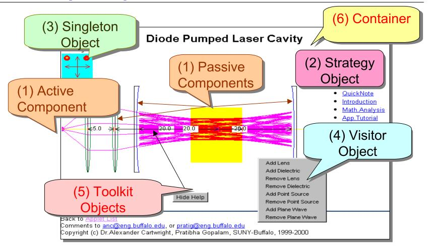
This Applet demonstrates a diode pumped laser system using ray tracing.
